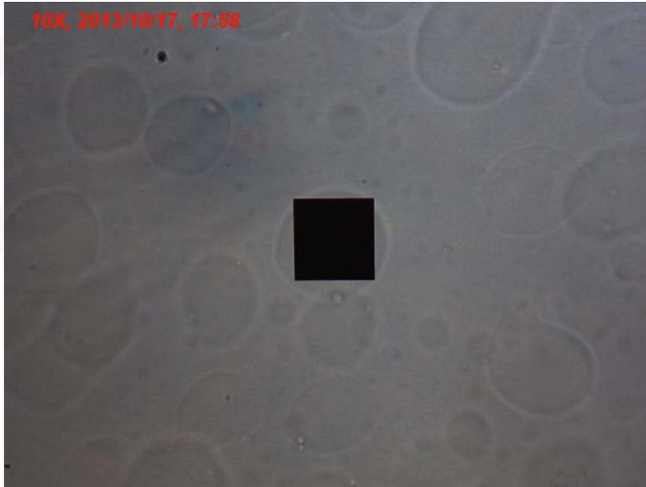
**Figure 1** Image from drop of 6% aqueous suspension of nanocrystalline cellulose. The black square in the center is the entrance aperture of the spectrophotometer.
