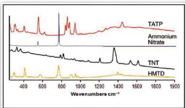
**Figure 6.** Unique Raman spectra of TATP, Ammonium Nitrate, TNT and HMTD.
