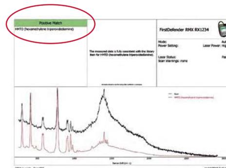
**Figure 5.** Analysis result with a positive identification of HMTD.
